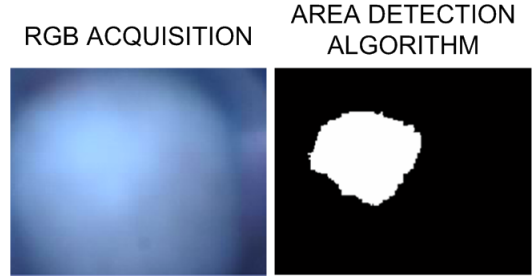
Figure 6: The results of the contact area detection algorithm: the RGB acquisition (on the left side) and the result of the final binarization (on the right side).
