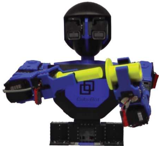
Fig. 1. The CubeBot, a 13 DOF VSA bi-manual torso, executing a peg-in-hole task. A pre-insert position is shown in the picture.
