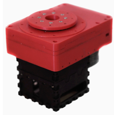
Fig. 1. Picture of the via actuator realized coupling a VSA-Cube and the Variable Damping add-on.
