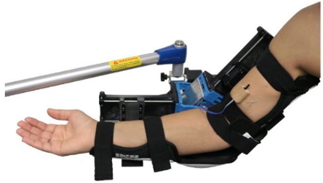
Fig. 1. FLExo , a 1DoF upper limb exoskeleton based on human muscle dynamics analogy.
