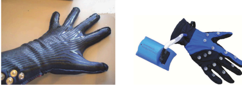
Figure 2: Examples of sensorized gloves. On the left, a sensing glove based on conductive elastomer sensor strips printed on fabric, each measuring a linear combination of joint angles [Tognetti et al., 2006]. On the right, the Humanglove (image courtesy by Humanware s.r.l. ( www.hmw.it/ )), using individual joint angle Hall effect sensors. Depending on the level of cross-talk between joint angles and measurements, this device can result in either a coupled or uncoupled model.
