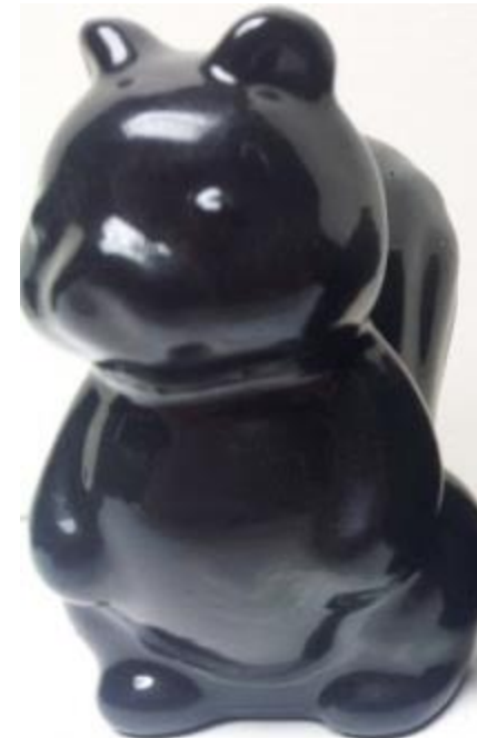
0.35 mm Layer Height with Vapor Bath Treatment
