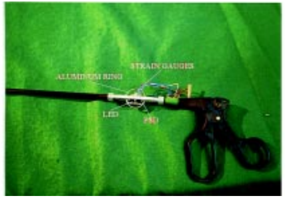
Fig. 7. Photograph of a sensorized laparoscopic forceps.
