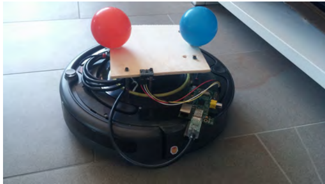
Fig. 1. Roomba robot equipped with front red marker and back blue marker mounted at 10cm.
